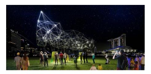
(ultra) light network exposes nature's basis as networks of energy and information flows and portrays the duality of light as luminous energy and light as immaterial quality. An ultra-light structure floats 2.5m overhead, consisting of 150 organic-shaped 3D printed nodes connected into a volumetric mesh. The presence of activity near the structure triggers dynamic patterns of light that pick up in intensity as more people approach the structure.
